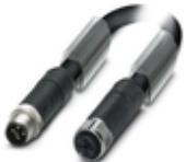
Power cable, 4-position, PUR halogen-free, black-gray RAL 7021, Plug straight M12, coding: T, on Socket straight M12, coding: T, cable length: 2 m, For direct current up to 12 A/63 V
