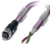
Bus system cable, PROFIBUS (12 Mbps), 2-position, PUR halogen-free, violet RAL 4001, shielded, free cable end, on Socket straight M12 SPEEDCON, coding: B, cable length: Free input (0.2 ... 40.0 m)
