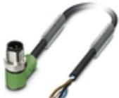
Sensor/actuator cable, 4-position, Variable cable type, Plug angled M12 SPEEDCON, coding: A, on free cable end, cable length: Free input (0.2 ... 40.0 m)
