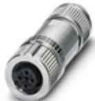
Connector, Universal, 5-position, shielded, Socket straight M12, Coding: B, Push-in connection, knurl material: Zinc die-cast, nickel-plated, external cable diameter 4 mm ... 8 mm
