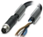
Power cable, 4-position, PUR halogen-free, black-gray RAL 7021, Plug straight M12, coding: T, on free cable end, cable length: 1 m, For direct current up to 12 A/63 V
