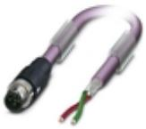
Bus system cable, PROFIBUS (12 Mbps), 2-position, PUR halogen-free, violet RAL 4001, shielded, Plug straight M12 SPEEDCON, coding: B, on free cable end, cable length: Free input (0.2 ... 40.0 m)
