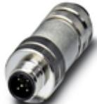
Data connector, PROFIBUS, INTERBUS, 5-position, shielded, Plug straight M12, Coding: B, Screw connection, knurl material: Zinc die-cast, nickel-plated, cable gland Pg9, external cable diameter 6.5 mm ... 8.5 mm
