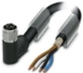
Power cable, 4-position, PUR halogen-free, black RAL 9005, shielded (Advanced Shielding Technology), free cable end, on Socket angled M12, coding: T, cable length: 1.5 m, For direct current up to 12 A/63 V
