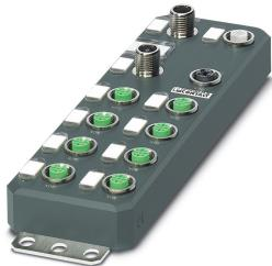
Axioline E, Digital I/O device, PROFIBUS DP, M12 fast connection technology, Digital inputs: 8, 24 V DC, connection method: 4-conductor, Digital outputs: 8, 24 V DC, 500 mA, connection method: 3-conductor, Plastic housing, degree of protection: IP65/IP67
