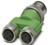
Y distributor, 4-position, Plug straight M12 SPEEDCON, coding: A, on Socket straight M8, coding: A and Socket straight M8, coding: A
