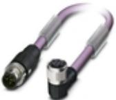
Bus system cable, PROFIBUS (12 Mbps), 2-position, PUR halogen-free, violet RAL 4001, shielded, Plug straight M12 SPEEDCON, coding: B, on Socket angled M12 SPEEDCON, coding: B, cable length: Free input (0.2 ... 40.0 m)
