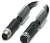
Power cable, 4-position, PUR halogen-free, black-gray RAL 7021, Plug straight M12, coding: T, on Socket straight M12, coding: T, cable length: 0.6 m, For direct current up to 12 A/63 V
