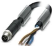
Power cable, 4-position, PUR halogen-free, black-gray RAL 7021, Plug straight M12, coding: T, on free cable end, cable length: 10 m, For direct current up to 12 A/63 V
