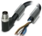
Power cable, 4-position, PUR halogen-free, black-gray RAL 7021, Plug angled M12, coding: T, on free cable end, cable length: 2 m, For direct current up to 12 A/63 V
