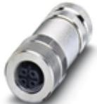
Data connector, PROFIBUS, INTERBUS, 5-position, shielded, Socket straight M12, Coding: B, Screw connection, knurl material: Zinc die-cast, nickel-plated, cable gland Pg9, external cable diameter 6.5 mm ... 8.5 mm
