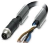
Power cable, 4-position, PUR halogen-free, black-gray RAL 7021, Plug straight M12, coding: T, on free cable end, cable length: 5 m, For direct current up to 12 A/63 V
