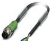
Sensor/actuator cable, 5-position, Variable cable type, Plug straight M12 SPEEDCON, coding: A, on free cable end, cable length: Free input (0.2 ... 40.0 m)
