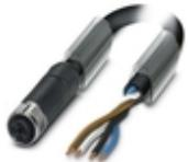
Power cable, 4-position, PUR halogen-free, black-gray RAL 7021, free cable end, on Socket straight M12, coding: T, cable length: 5 m, For direct current up to 12 A/63 V
