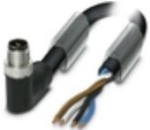
Power cable, 4-position, PUR halogen-free, black-gray RAL 7021, Plug angled M12, coding: T, on free cable end, cable length: 5 m, For direct current up to 12 A/63 V
