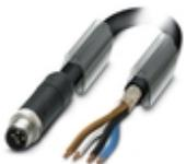
Power cable, 4-position, PUR halogen-free, black RAL 9005, shielded (Advanced Shielding Technology), Plug straight M12, coding: T, on free cable end, cable length: 1.5 m, For direct current up to 12 A/63 V
